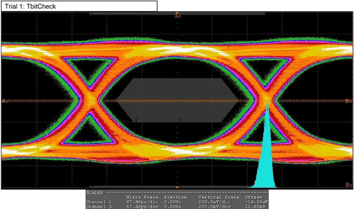
✓ 7-10: D2 - Mask Test Reference: Test ID 7-10
