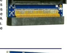
Analyzer to Mictor probe. It enables use of legacy Mictor connector based logic analyzer probe such as E5346A E5380A P6434. The  $\underline{\sf ZX132AAM}$  is designed in 4 layers
