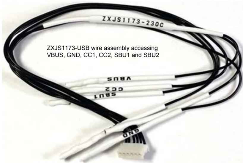
ZXJS1173-USB wire assembly accessing VBUS, GND, CC1, CC2, SBU1 and SBU2
