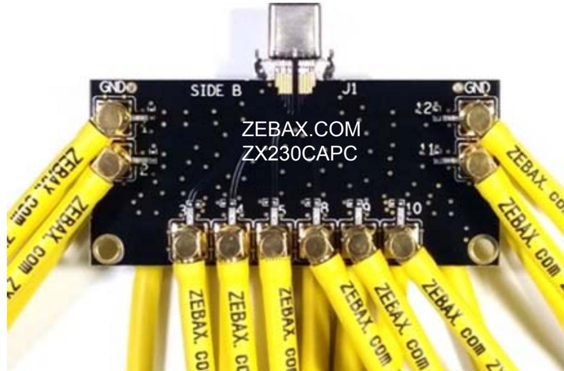
**SMA Cable Assembly** is semi-flexible coax cable with maximum bends of 35mm. Please do not over exert beyond the cable's tolerance.
