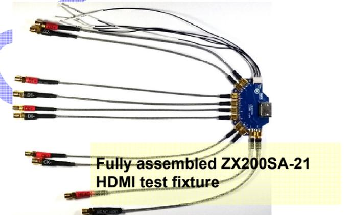
**SMA Cable Assembly** is semi-flexible coax cable with Max. bends of 35mm. Please do not over exert beyond the cable's tolerance.
