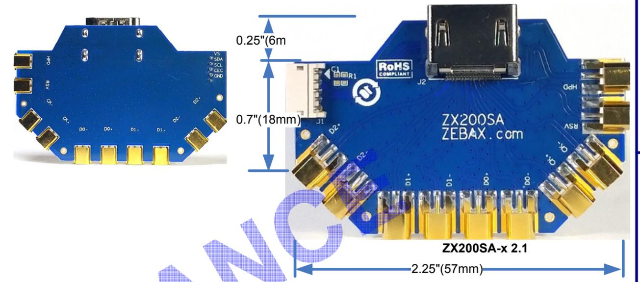
ZX200SA-21 is offered supporting HDMI Type A Plug connector.
