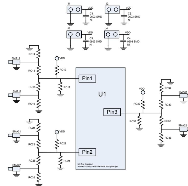
**Stuffing option, Matrix :** Table below provides suggested stuffing options for the DASS components for push-pull, and open drain devices for INPUT, OUTPUT, supply and the GND signal interfaces.
