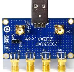
ZX230AP Type A Plug USB Test Fixture S-Parameter
