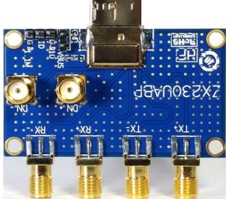
ZX230ABP Type AB Plug USB Test Fixture S-Parameter
