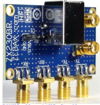
ZX230BR Type B Receptacle USB Test Fixture S-Parameter
