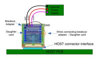
GND test point is common to all Zebax Breakout adapters, check connector type for GND connection at connector or requiring external GND interface. Wire interface such as Zebax accessory, part number  $ZX100ACC\mbox{-}SS6.$
