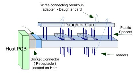
Figure 7 – Placing Daughter card on top of Breakout adapter, 3D side view – REMOVED headers, interfacing directly to Pads (Header landing pads).
