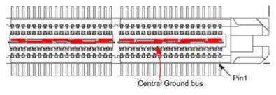
Figure 4- Mictor connector offering in Plug and Receptacle height - 0.26" (6.6mm) is commonly used
