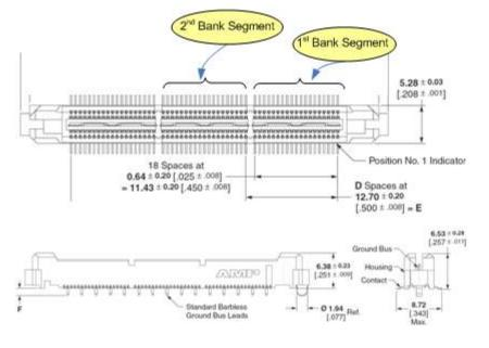
**Figure 5** – Mictor Connector Plug mechanical outline- bank segment
