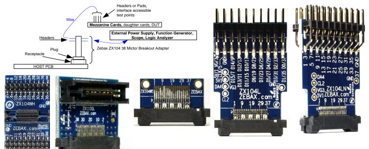
Figure 7 – Zebax ZX104x 38 Mictor Breakout adapter using Mictor Plug - typical applications
