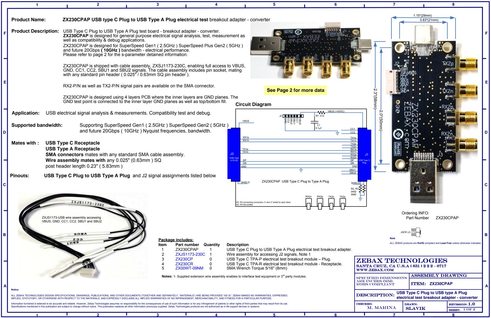
ZX230CPAP USB Plug type C to USB Type A Plug electrical test breakout adapter Cont's **Product Name:**
